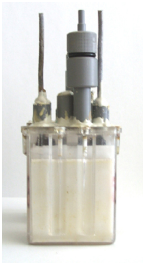
Fig. 1. Photograph of a 2 V/4.5 Ah test cell.
